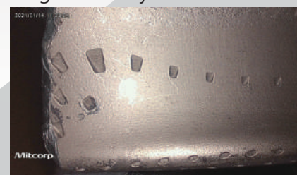
2560*1440 output by 6.0 mm HD probe (10 mm distance)
