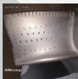
1600*1600 output by 3.9 mm HD probe (30 mm distance)
